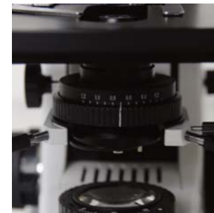
[5] Mechanism of centring the condenser
