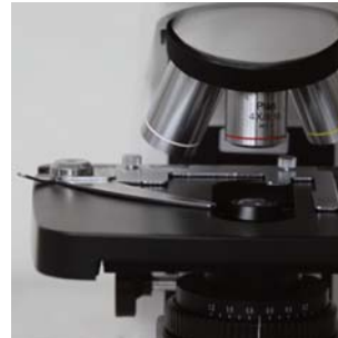
[3] Clamp that can hold up to two standard size slides at the same time
