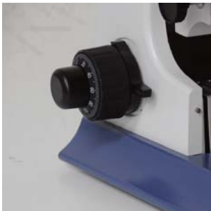
[1] Coaxial knobs for coarse and fine focusing adjustment
