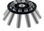
Angle rotor | GLH016 20 mL×12 5000 rpm/3800 ×g
