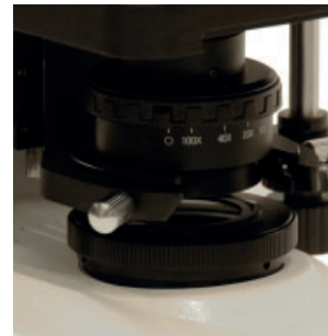
LED light system and condenser Abbe N.A. 1.25 with diaphragm type.
