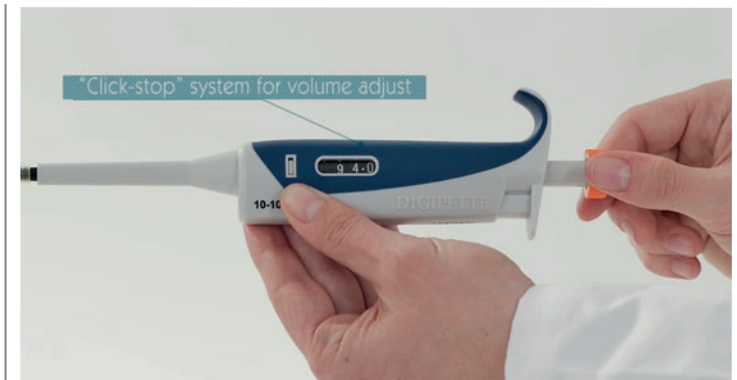
“Clik-stop” mechanism of volumen selection
