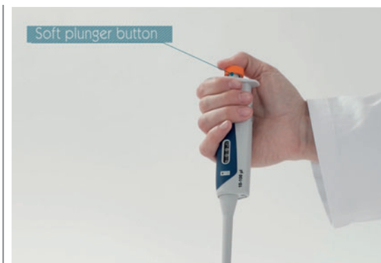
Smooth plunger mechanism
